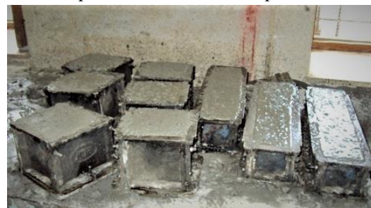
Fig 6: casting of samples (cubes and prisms)
