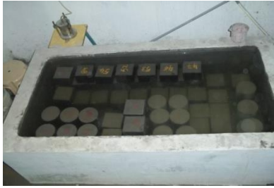
Fig 7: Curing of examples for 7 days, 14 days and 28 days age
