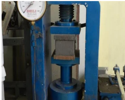
Fig 8: Testing of 10%MSW specimen at 7 days curing
