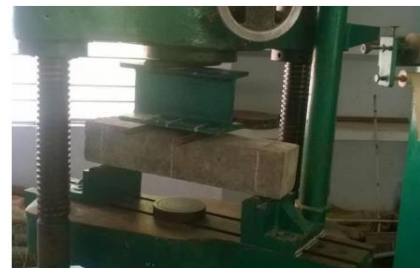
Fig 10: Flexural strength of prism specimen
